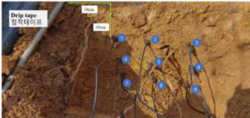
PG 1. soil moisture content measure sensors Installation by depth and distance
